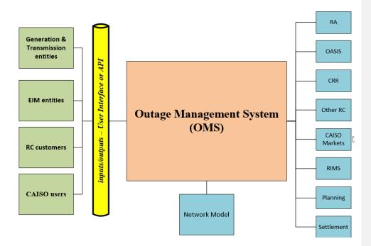
The OMS application is considered the primary interface for submission of outage information to the Long-Range, Short-Range, and Real Time outage processes that comprise the operations horizon, and serves as the conduit for the ISO CRR, RA, and RIMS processes.
